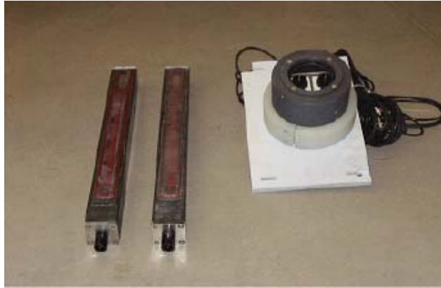
Figure 3. 171 kHz transducers and video camera.
