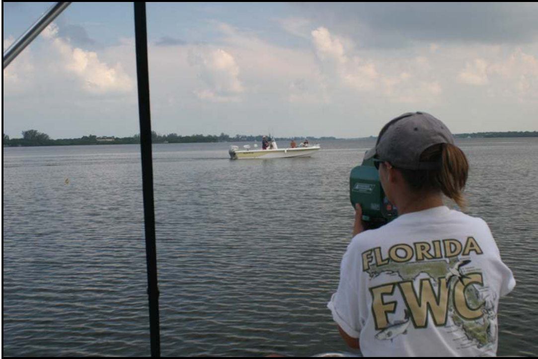
Figure 7. A laser range finder was used to collect distance and bearing to all vessels that passed the focal manatee under observation, identified by the floating GPS tag on the left side of the image.
