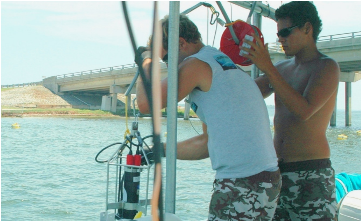
Figure 5a. Site-specific bathymetry, and sound speed profiles were measured using CTD casts from the boat.
