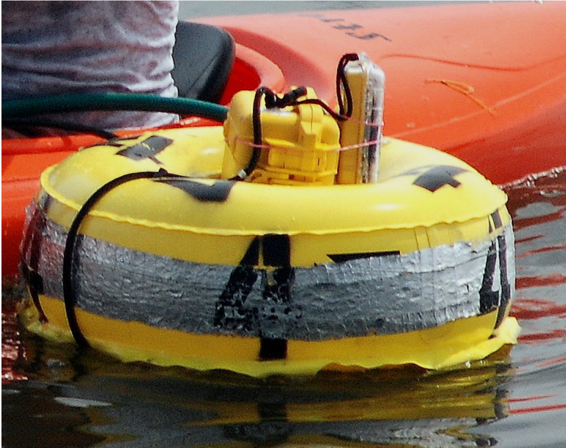
Figure 2b. Numbered buoys helped to grid areas visually as well as acoustically with both GPS and DARPs.
