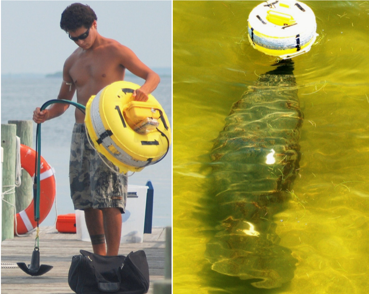
Figure 2c. The buoy anchoring system negated risks of possible entanglements with any curious manatees.
