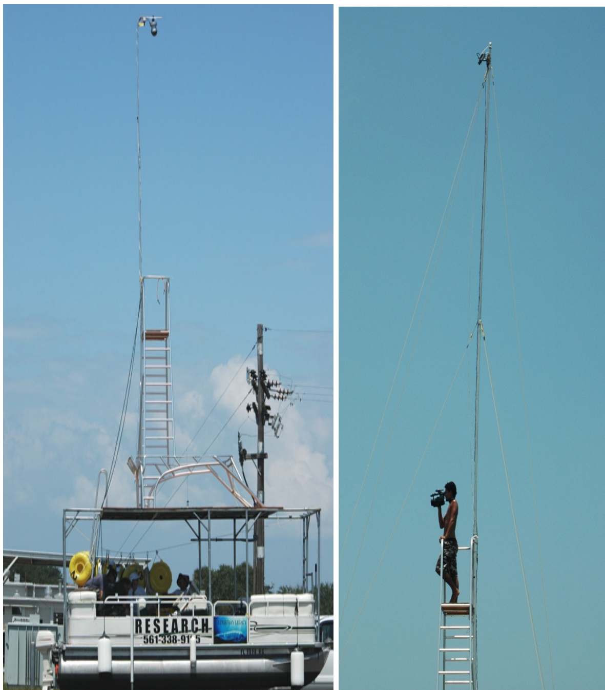
Figure 4a. Boat shown with RR engine, elevated viewing decks and 14m extended remote video camera.
