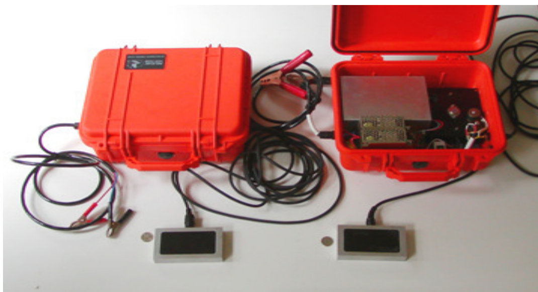
Figure 9a. SSB, combiner, power amplifier and acoustic projector.
