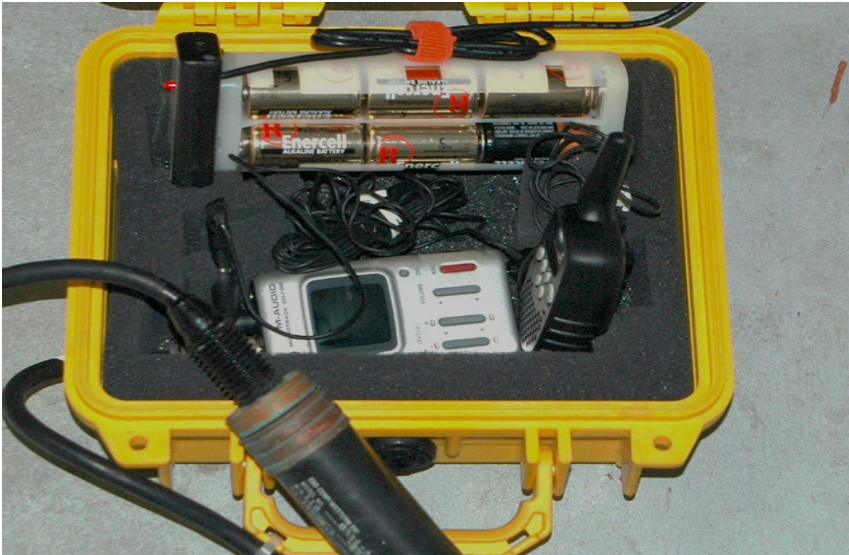
Figure 2a. DARP components: two channel digital flash card recorder, power sled, walkie talkie, microphone, and hydrophone.
