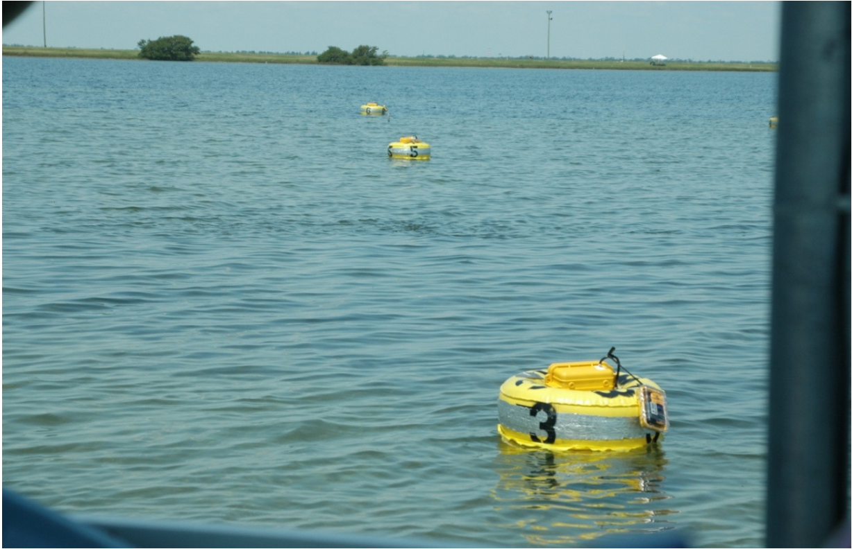
Figure 5b. Propagation (transmission loss) measurements were made using a calibrated USRD J9 projector directed along a line of instrumented buoys anchored at varying distances.
