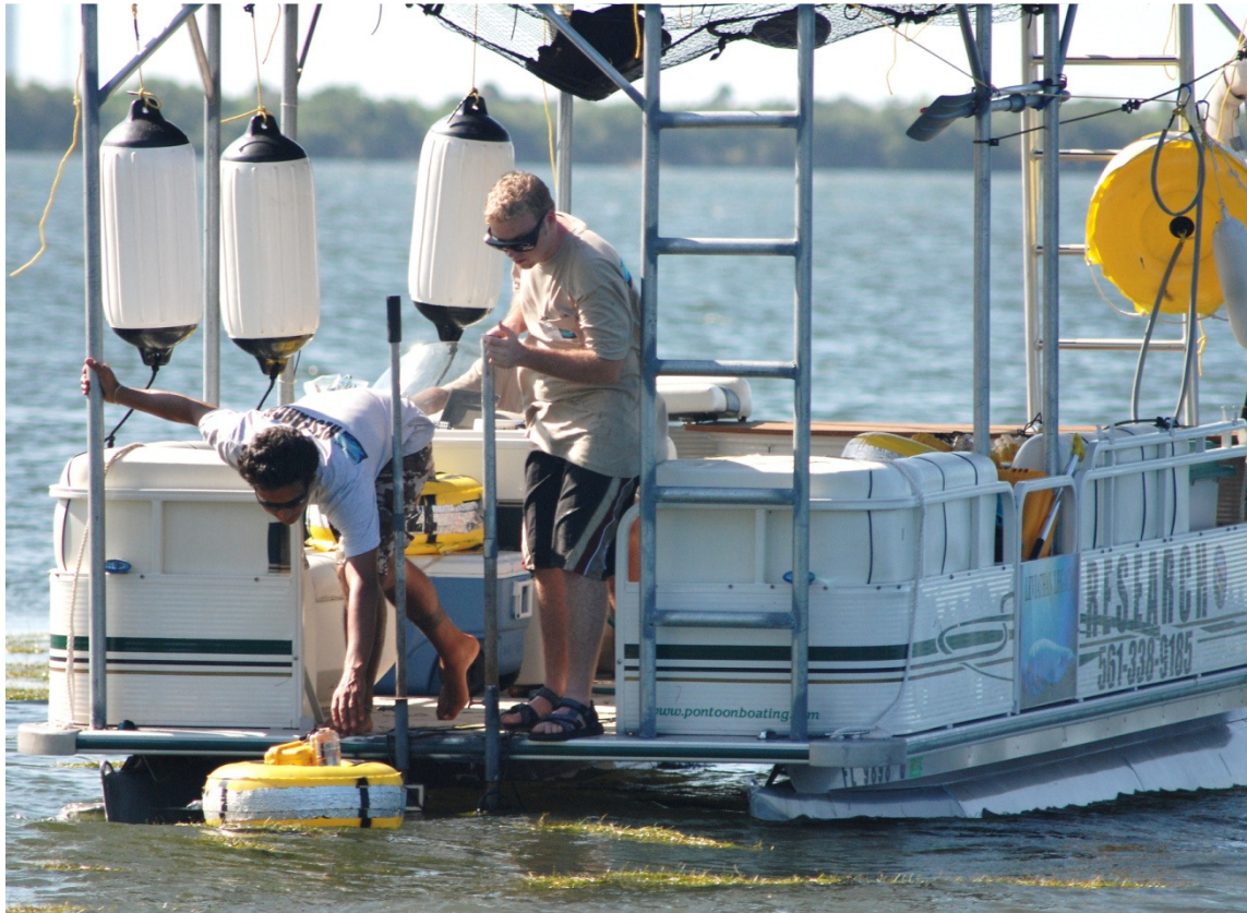
Figure 16. Setting a reference buoy for propagation measurements through sea grass mats and beds. Parametric and J-9 projectors were positioned at the middle of bow with the attachment poles seen here at the bow.
