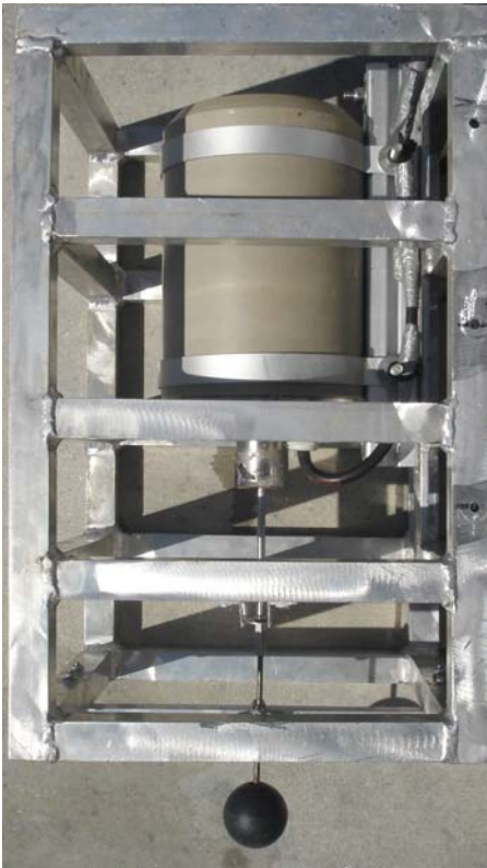
Figure 5. Dipole shaker with sphere mounted in the end. The ball contains a three-dimensional accelerometer that is used to measure the acceleration of the ball for each test frequency. The cage is used for mounting the shaker to the side of the tank and also protecting the shaker from the manatee.
