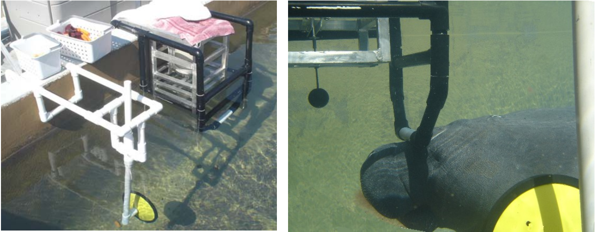
Figure 4 – Experimental setup showing the shaker with a black PVC stationing apparatus. The task of the manatee is to station on the black PVC (see photo on right) and then upon detecting the movement of the dipole to touch the yellow response paddle shown on the left.
