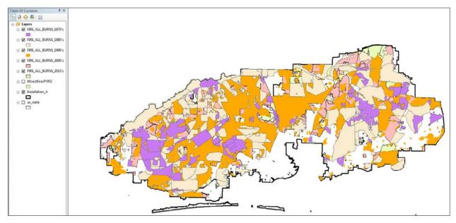
**Figure 9:** Test map of Eglin Air Force Base fire data created to verify spatial tables have valid geometry; this map would not appear correctly if the geometries were invalid.
