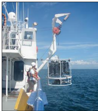
Rosette sampler with CTD and Niskin bottles being lowered for water collection
