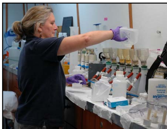
Sample filtration for analysis of chlorophyll a in seawater
