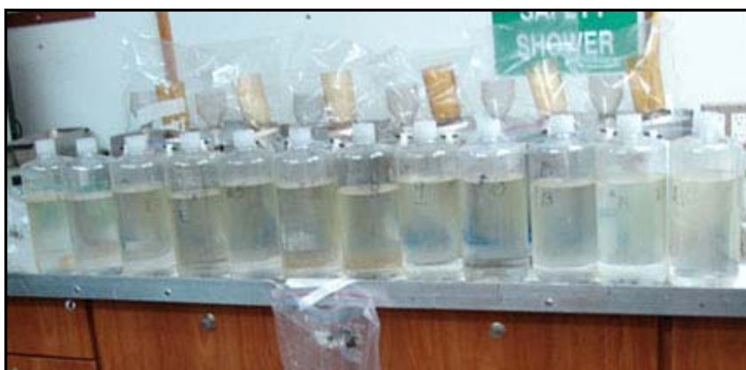
Experiment measuring nitrogen uptake by a Karenia bloom
