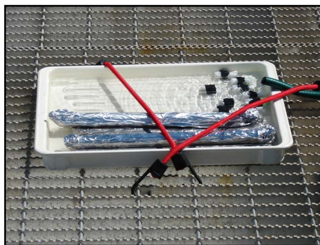
Photochemical experiment examining the role of ultraviolet light on producing nutrients from dissolved organic material
