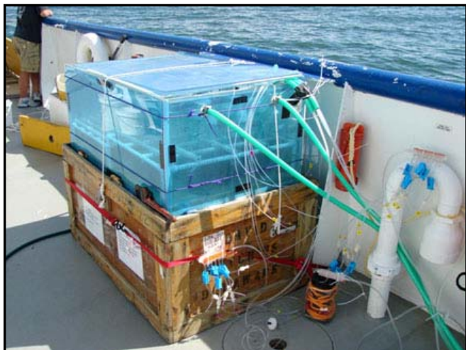
On-deck incubator for bioassay experiments examining the influence of changing carbon dioxide concentration on algal physiology
