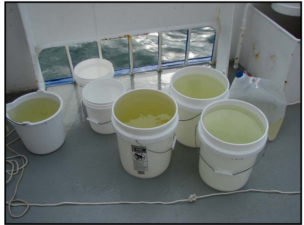
Water samples from different parts of Karenia bloom showing the influence of different concentrations on water color. Darker waters have the highest Karenia concentrations.
