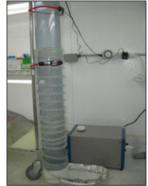
Experimental column wrapped in water-filled tubing attached to a chiller
