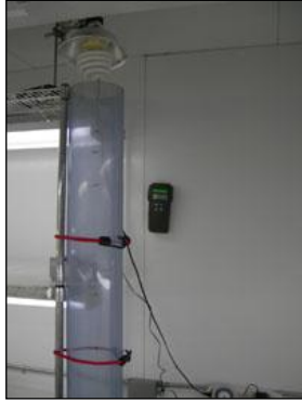
Experimental column to study vertical migration of Karenia brevis
