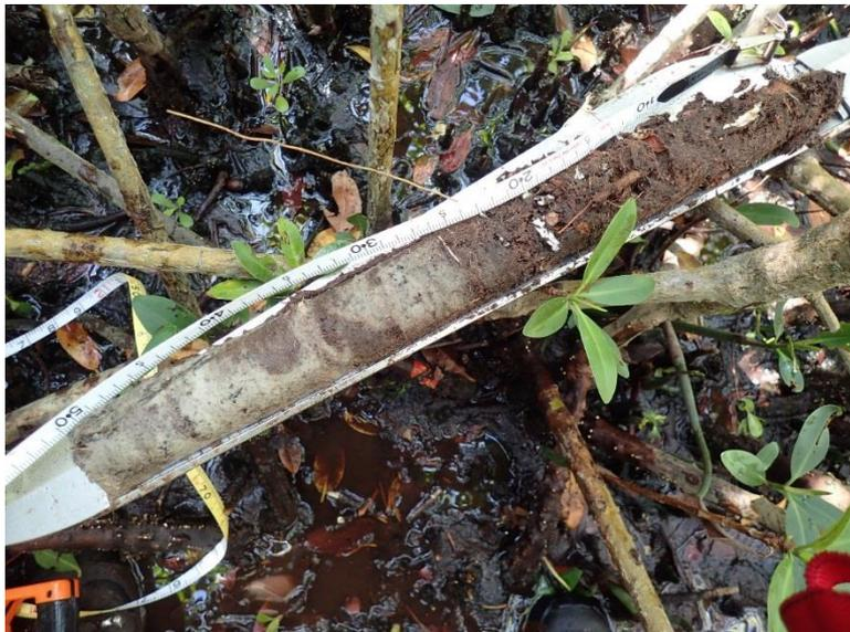
**Loss-on-ignition (LOI)** = staged combustion (550° C and 950° C) process to determine sedimentary organic carbon content:
