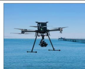
Inspired Flight's IF1200A UAV equipped with LiDAR USA's LiDAR unit used in this study.
