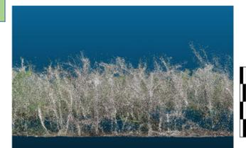
"True color" point cloud obtained from UAV photogrammetry data collected at the Imperial Shores site on 3/5/2023. These data were used to successfully measure tree heights in the analysis to the right.
