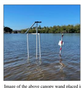
Image of the above canopy wand placed in Estero Bay. Data from the below canopy wand is compared to this wand to compute LAI.
