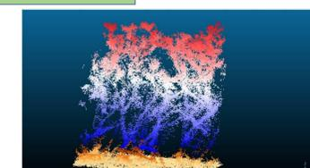
Subplot data were extracted from the point cloud on the left and LAI was computed using a model from the literature using additional data.
