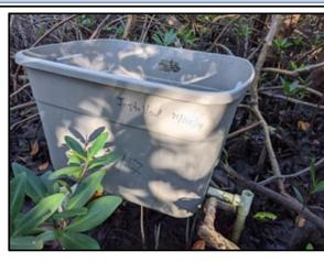
Litter traps used for collection of litterfall data for comparison against remote sensed LAI (leaf area index) data.
