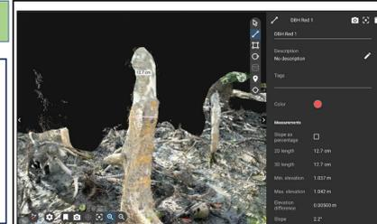
The viDoc RTK rover system has shown promise for mapping and measuring DBH at our site. While processing time is a limitation, the data collection speed significantly reduces time in the field where heat stress can be problematic for researchers. Measurement accuracy appears similar to *in situ* DBH tape measurements. Unfortunately, satellite signal strength may be a limiting factor for the RTK unit in dense mangrove canopy systems.
