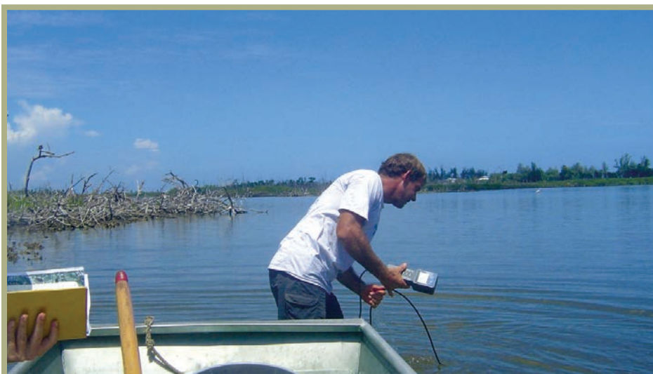
Figure 23. Using handheld instrumentation to measure water temperature and salinity.
