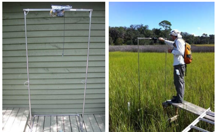
Figure 1.15. Assembled lightweight camera stand for close-to-earth remote sensing (left) and acquisition of nadir images (right). Photo credit: GTMNERR
