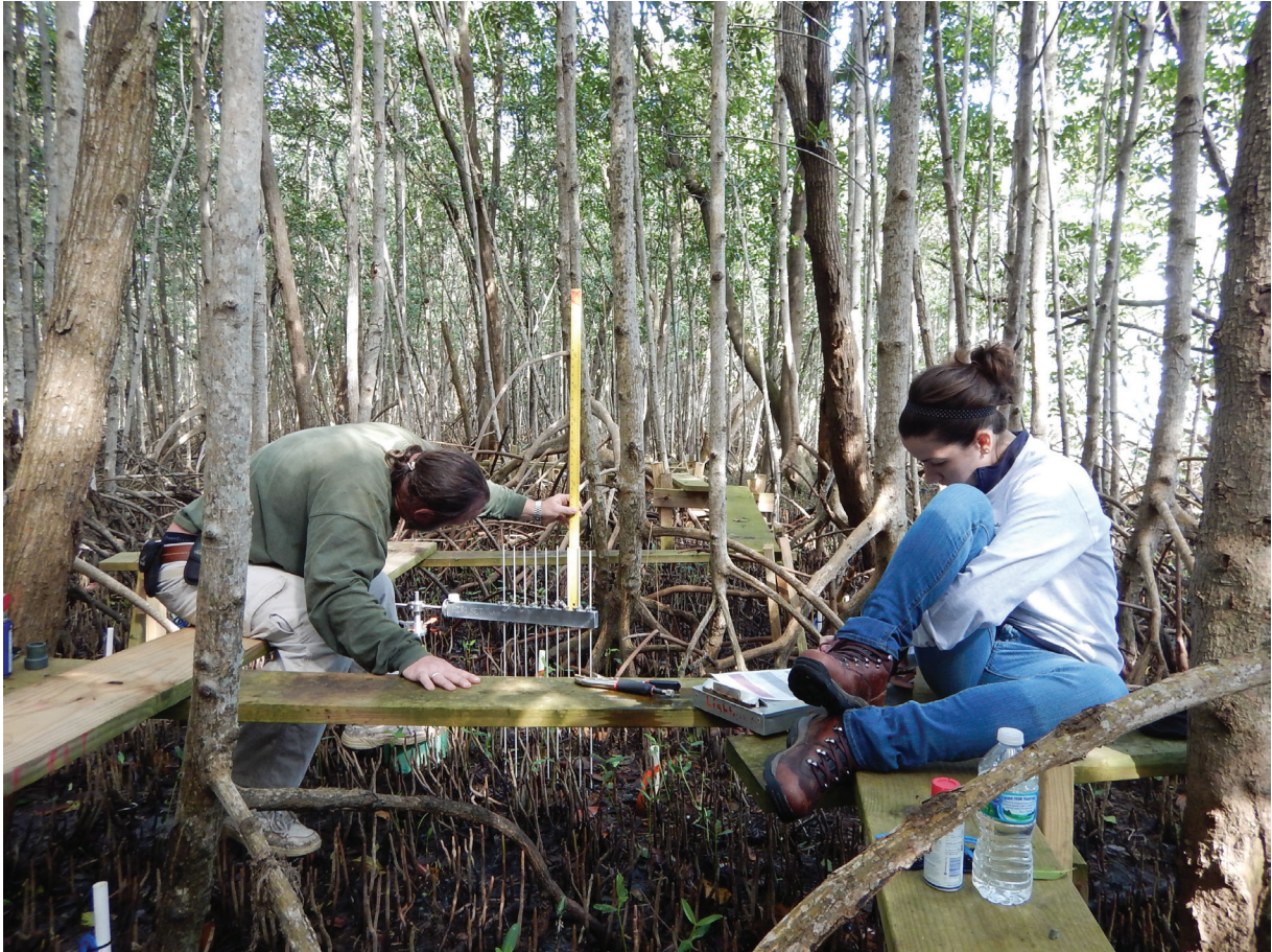
Figure 10.5. Kevin Whelan, SFCN ecologist, measures soil surface elevation using a surface elevation table (SET). The SET is attached to a permanent benchmark. The height of the pins transcribes the elevation of the soil and standardizes it to a fixed reference point on the horizontal metal arm. Repeated measurements over time are used to monitor the rate of change in soil elevation.
