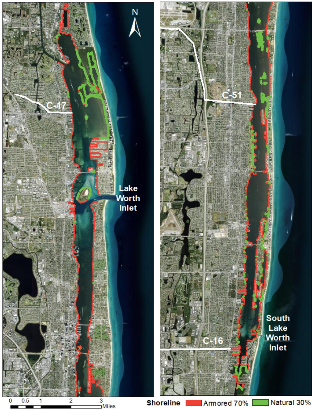
Figure 11.3. Lake Worth Lagoon shoreline characterization. Red represents armored shorelines (70%) and green shows where natural shorelines remain (30%). Data source: LWLI 2021.
