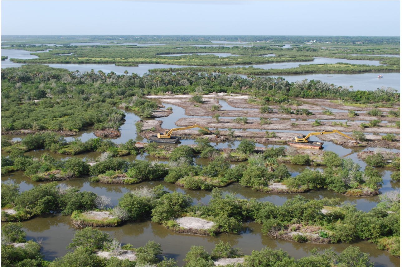
Figure 12.8. Coastal wetlands in Mosquito Lagoon that were ditched with a dragline in the late 1960s to control mosquitoes. The foreground shows the results of the original ditching; restoration is under way in the center of the image. Photo credit: Linda Walters, University of Central Florida.
