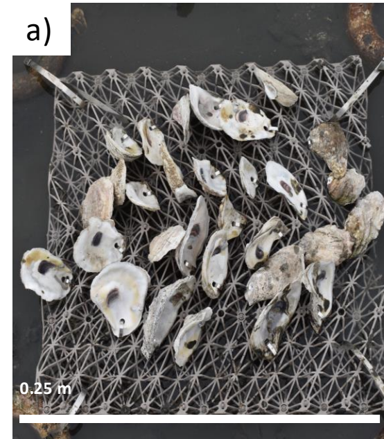
a) BESE-elements ® mat and b) Jute fiber
