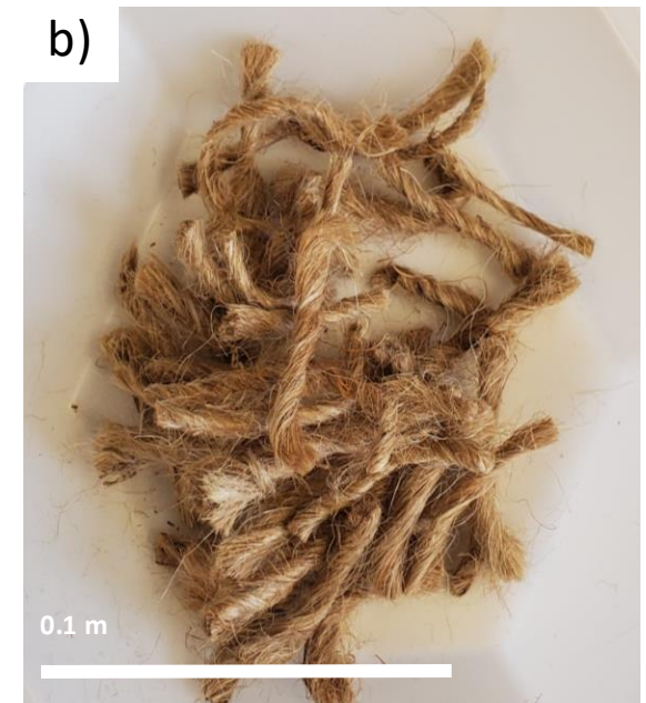
a) BESE-elements ® mat and b) Jute fiber
