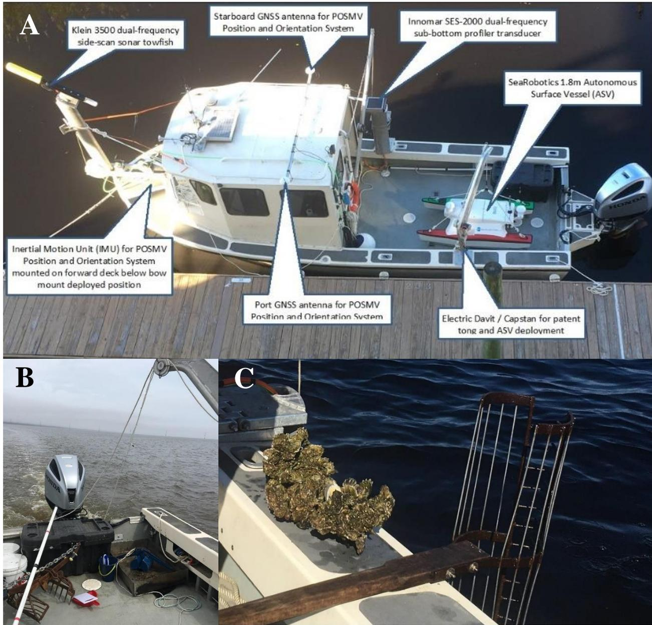
**Figure 3.** A: *R/V Diversity* (24-foot length, 8-foot beam) with major components used in acoustic surveys labeled: Klein 3500 side-scan sonar deployed from a bow mount; Innomar SES-2000 dual-frequency parametric sub-bottom profiler mounted amidships; Applanix POSMV GNSS antennae mounted on both sides of wheelhouse; SeaRobotics ASV; and davit for deployment of ASV and patent tongs. B: gear used for bottom sampling (ground-truthing); C: handheld tongs.
