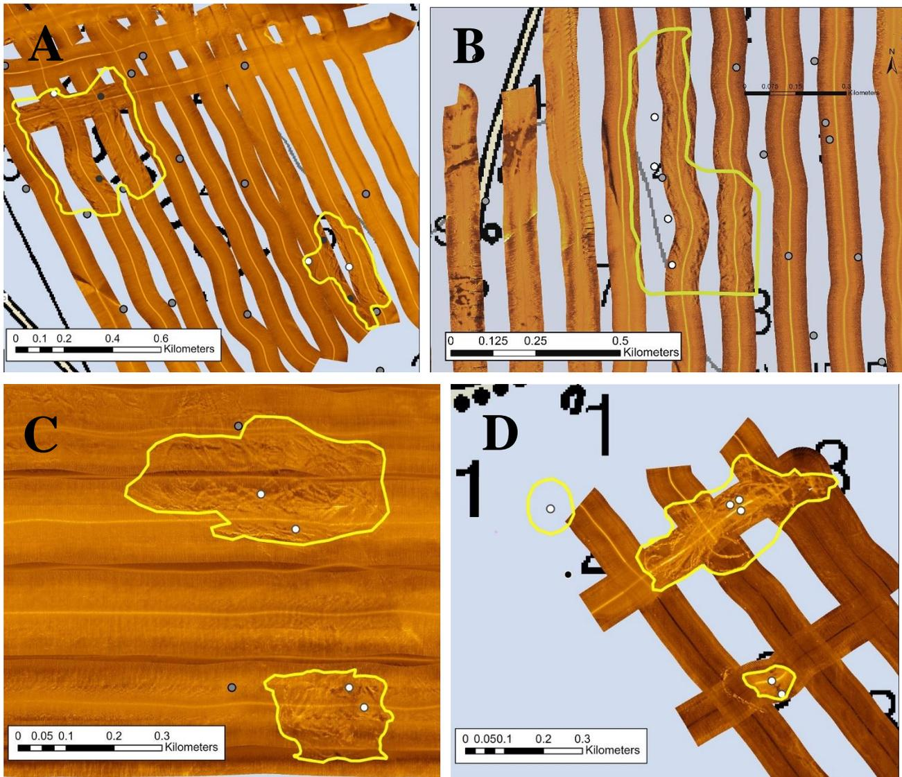
**Figure 10.** Composite of images illustrating how side-scan imagery was used in combination with ground-truthing data to determine spatial extent of live oyster reefs. A: Bulkhead bar area; B: Cat Point bar; C: Hotel bar; and D: restoration site in St. Vincent Sound.
