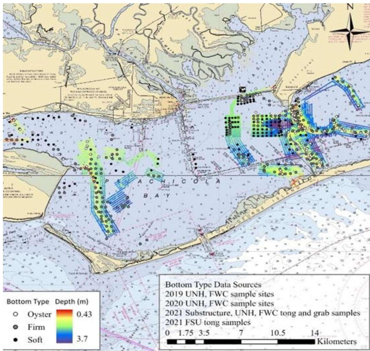
**Figure 7.** Bay-wide single-beam bathymetric data (water depth in meters) with ground-truthing data overlaid
