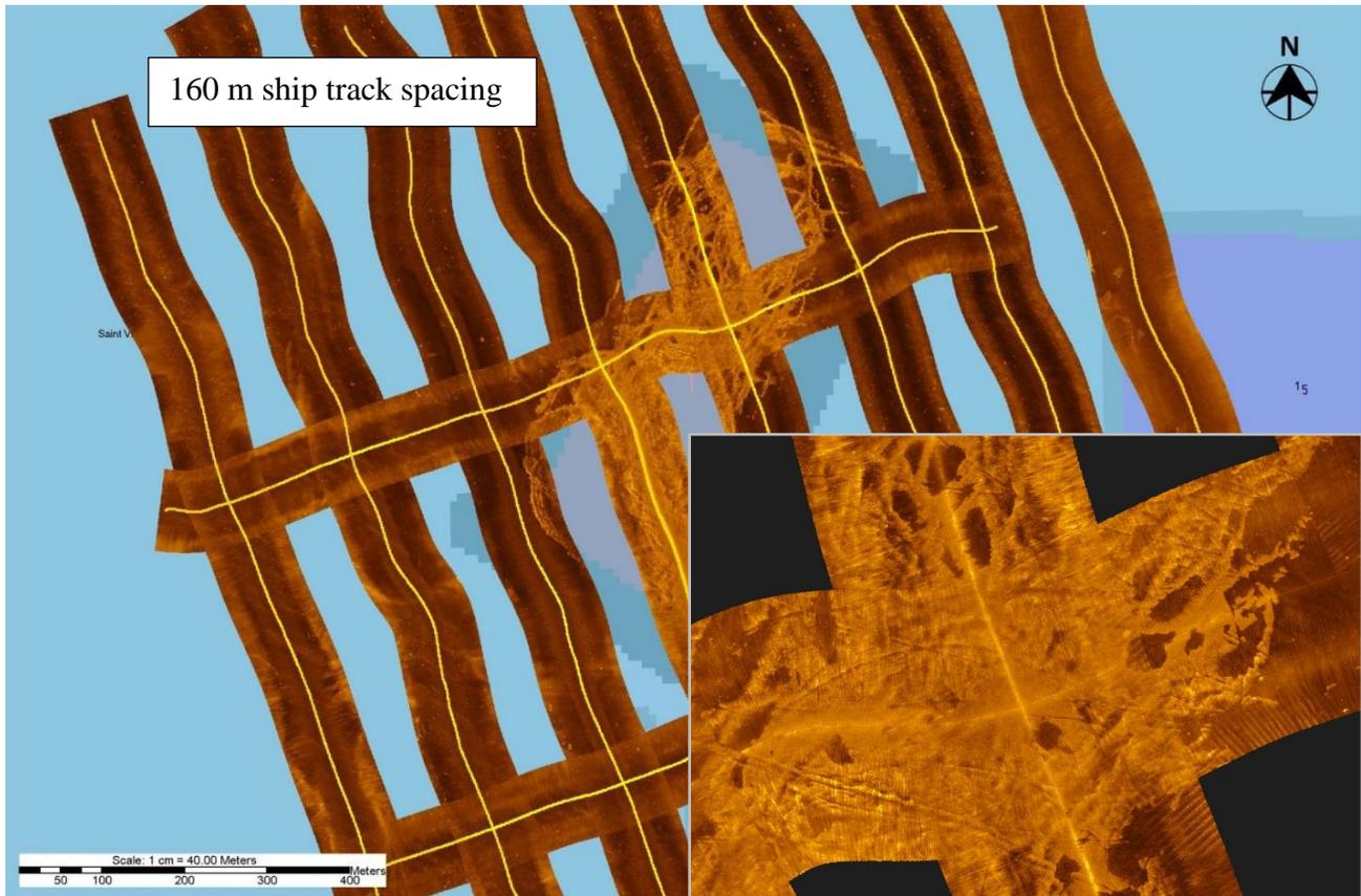
**Figure 9.** Side-scan sonar mosaic and single-beam trackline bathymetry from northern St. Vincent Bar area. Note details of cultch material on the bottom of restoration area indicated by faint jagged-edged rectangle on base map. The inset zoomed-in view around a crossline junction illustrates the sporadic nature of the rock placement and also highlights the stark acoustic contrast between the high-reflectance rock and oysters and the underlying low reflectance muddy sediment.
