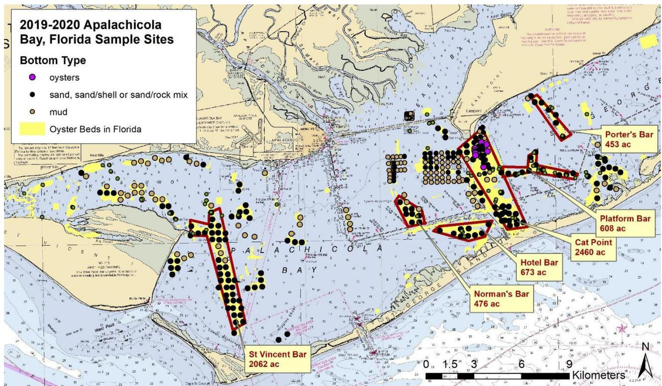
**Figure 6.** Bottom types (ground-truthing data) based on UNH and FWC sampling in 2019 (Grizzle et al. 2020) and 2020 in areas previously mapped as oyster reefs. Red polygons indicate the initial target areas for acoustic surveys.
