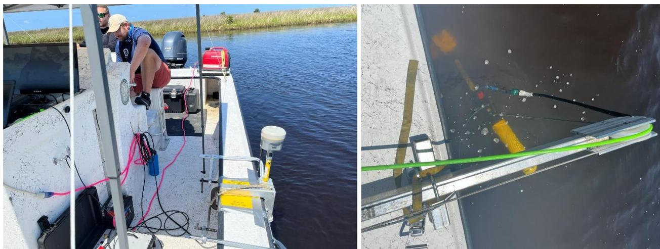
**Figure 4.** Custom gear for deploying acoustic sensors from FWC vessel. Left: single-beam sonar and GNSS. Right: bow boom for Klein side-scan tow fish.
