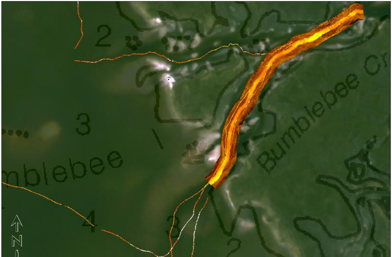
Figure 4. Acoustic survey data from Bumblebee Creek comparing the initial reconnaissance single-beam track line bathymetry (narrowest shiptracks) and multibeam imagery. The full multibeam 2D (side-scan) imagery swath was 100m (50m per side), while the full multibeam 3D bathymetry swath was generally limited to about eight times the water depth (or ~25m in 3m of water).
