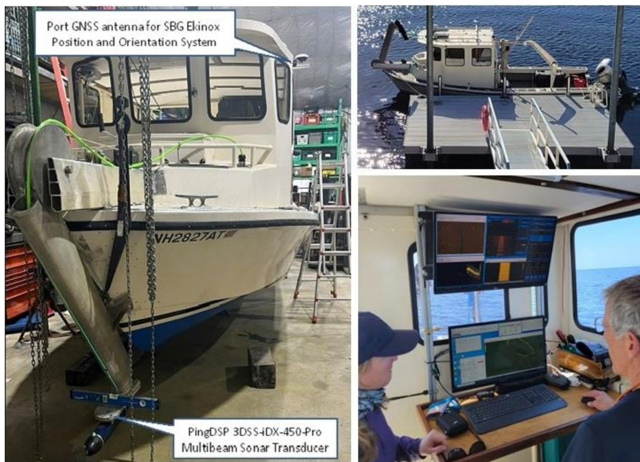
Figure 3. Left: Acoustic gear on Substructure's Diversity with bow-mount and towfish in deployment position. Top: Diversity with bow-mount in raised position. Lower: Sonar monitors in wheelhouse.
