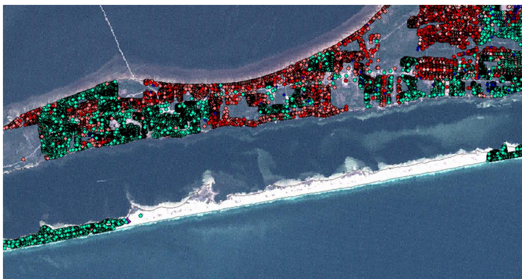
Figure 8: Gulf Breeze, FL parcels on central sewer system (green dots) and septic systems (red dots)
