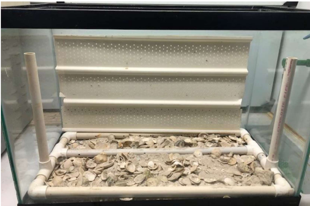
Figure 7: Small scale version of a PVC under-gravel filtration system in a 20-gallon aquarium.
