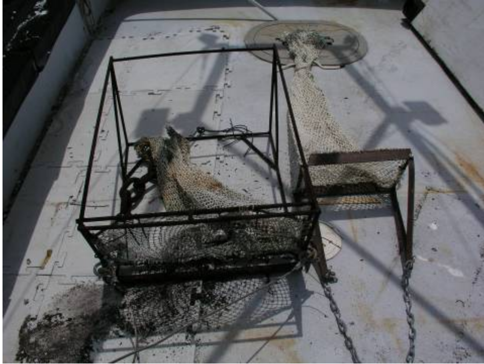
Figure 5. Dredges used in this study: 0.69 x 0.50 m (left) or 0.42 x 0.25 m (right).
